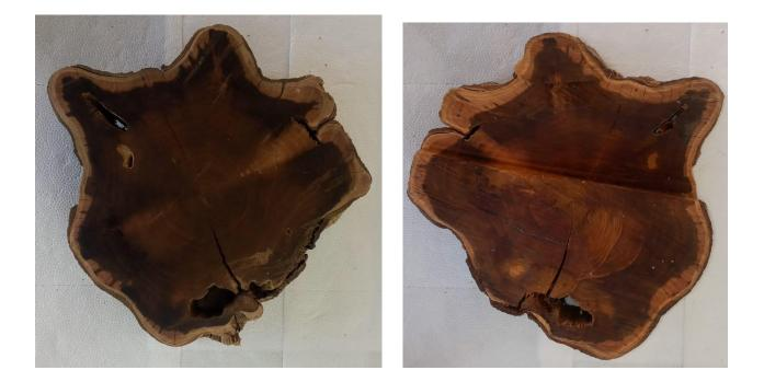
Similarly we can observe in the two photos below that the cross-section of this tree, also 31 years old, presents sapwood with a thickness of approximately 2 centimetres, but even so, the heartwood is well developed. We observe that this trunk also presents buttresses, indicating a different variety.
